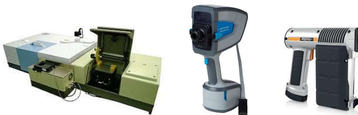
Novel indicator technologies (left to right): a laboratory MIR spectrometer, a portable field MIR spectrometer and a portable XRF analyser.
